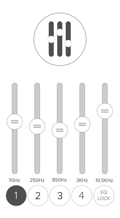
Customize your sound with the Minirig EQ, pick the frequency you would like to turn up or turn down and simply move the slider to where you want it to be.
